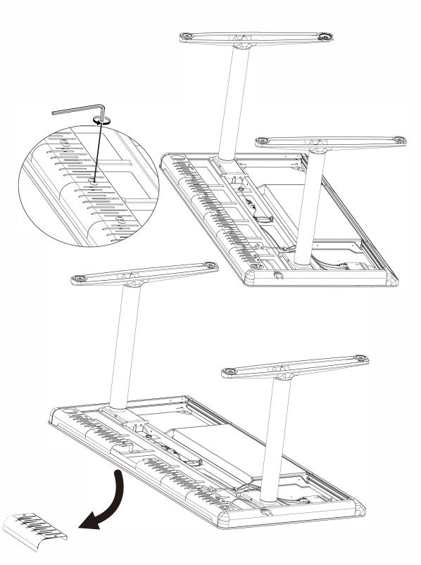
The cable management can be opened in this way to put sockets and electric wires
