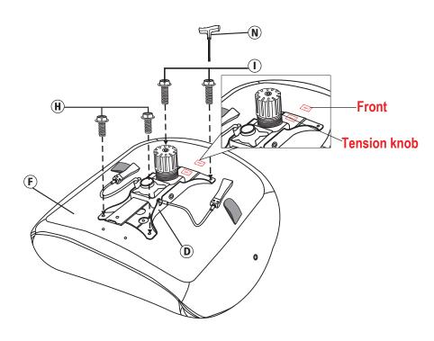
Align the Back Cushion (G) with the Seat Cushion (F) by positioning the back support plate over the Seat Plate (D) with 1-1/4" Screws (I).
